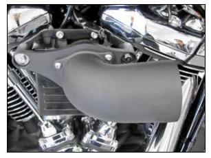
10. Install the intake tube onto the base plate. **NOTE: Apply one drop of the provided thread locker to the threads of each bolt.**
