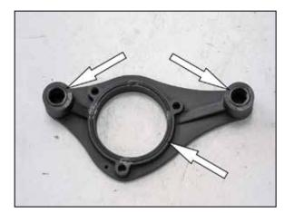
7. Install two of the breather O-rings and the throttle body O-ring into the base plate as shown. NOTE: Use a few small dabs of grease to secure the O-rings in place while installing the base plate to the engine.
